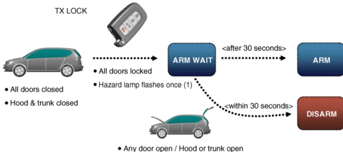
※ Remark: For a vehicle equipped with Smart Key system, the same process is applied to Passive door lock function.
