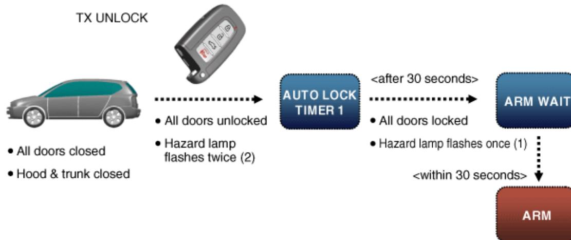
※ Remark: For a vehicle equipped with Smart Key system, the same process is applied to Passive door lock function.
