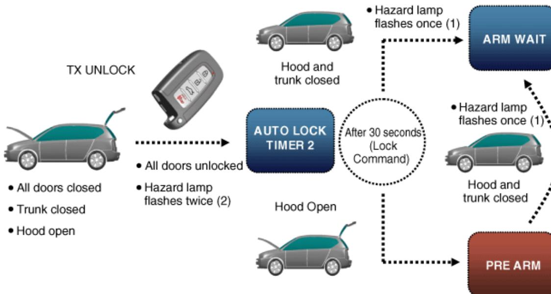
※ Remark: For a vehicle equipped with Smart Key system, the same process is applied to Passive door lock function.
